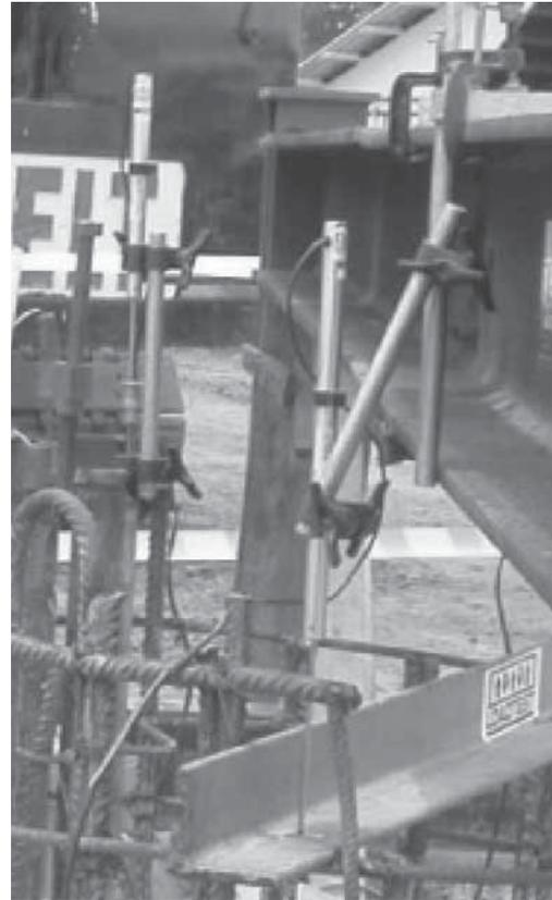
Figure 5. Two LVDTs: one monitoring the top of pile from the reference beam and the pile compression above the O-cell.
