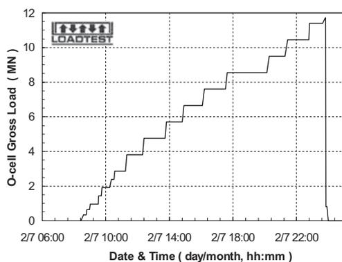
Figure 6. O-cell load increment—time plot.
