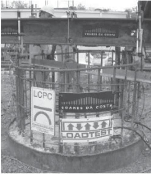
Figure 7. Pile Head with instrumentations.
