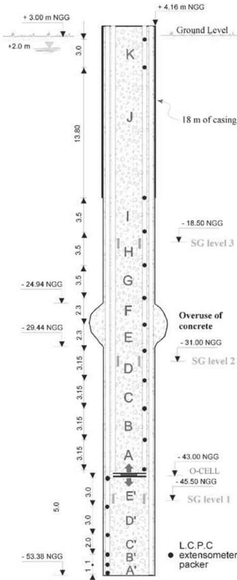
Figure 4. Schematic section of the test pile.
