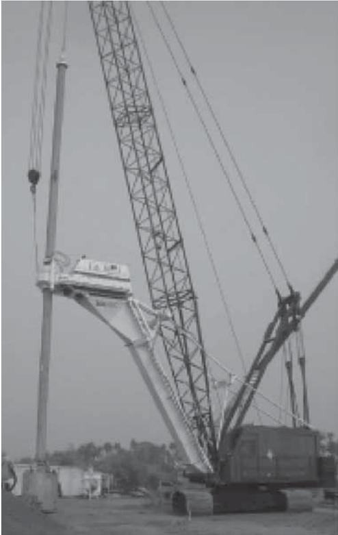
Figure 1. Link Belt LS-418 with Soilmec RT3-ST.
