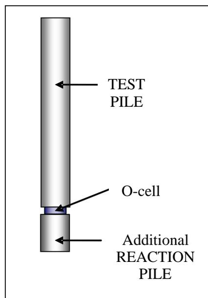
**Fig. 8** Illustration of O cell arrangement for a push-out test
