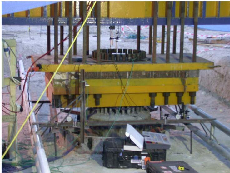
**Fig. 6** Pile head requirements on a 10 MN pull out test
