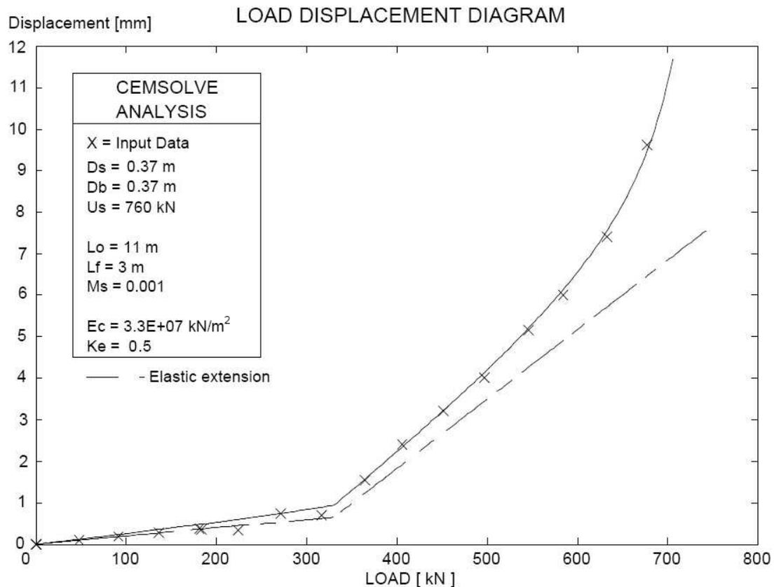
Fig. 4 Driven pile tension test and Cemsolve Analysis
