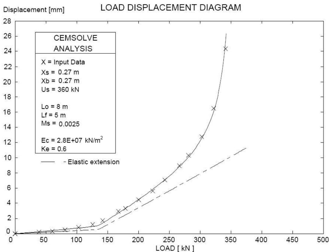
**Fig. 3** Precast 270 mm square -Tension test and Cemsolve Analysis.
