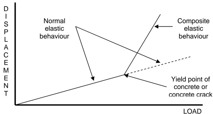
**Fig. 1** Change of elastic modulus with tension load in reinforced concrete
