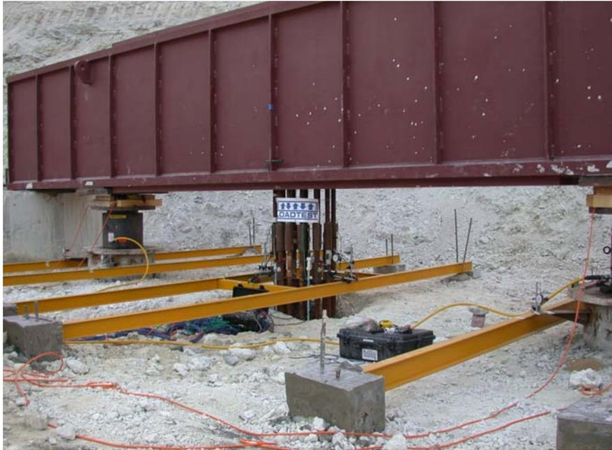
**Fig. 7 Pile head requirements on a 18 MN pull out test**
