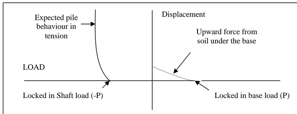
**Fig. 10 Locked in forces after loading and resulting upward friction available**
