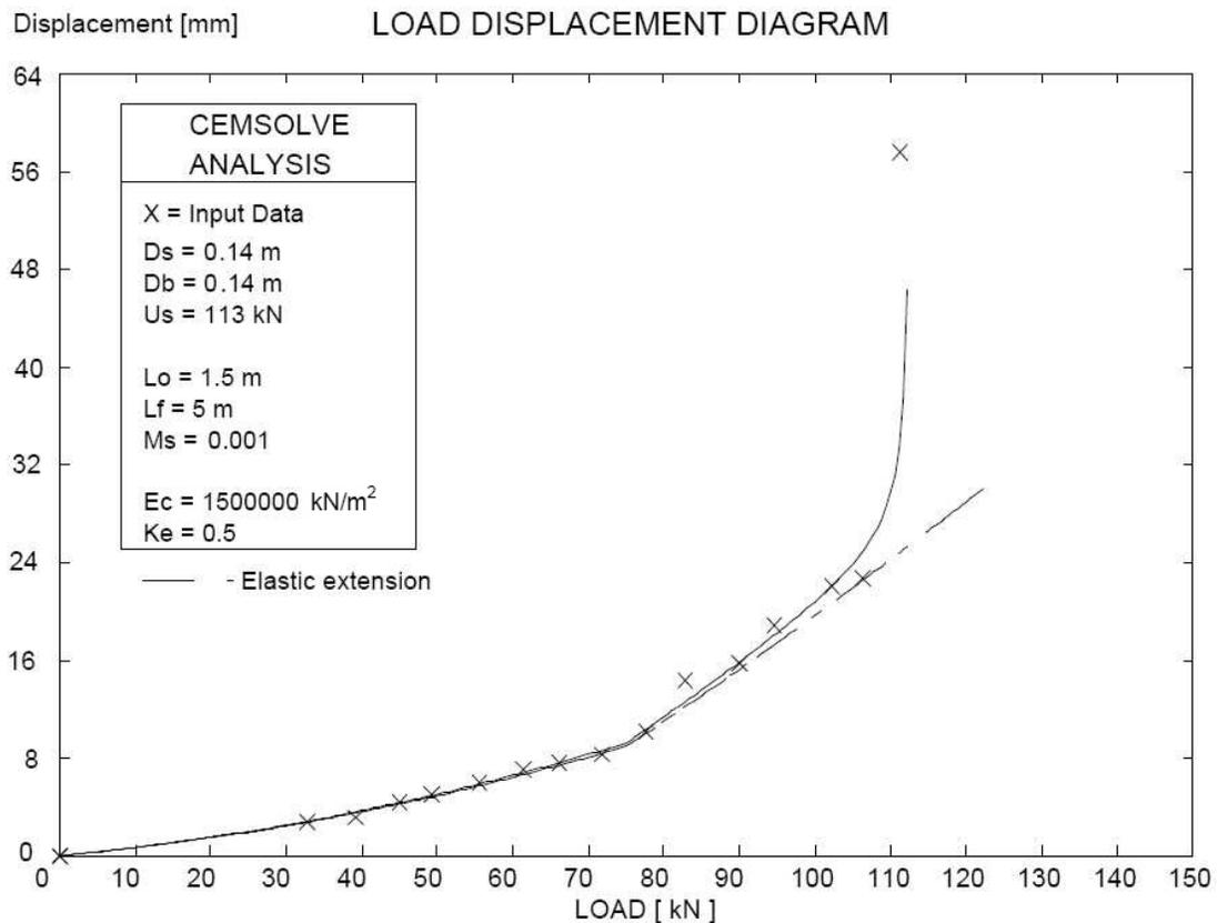
**Fig. 2** Anchor tension test results and Cemsolve Analysis
