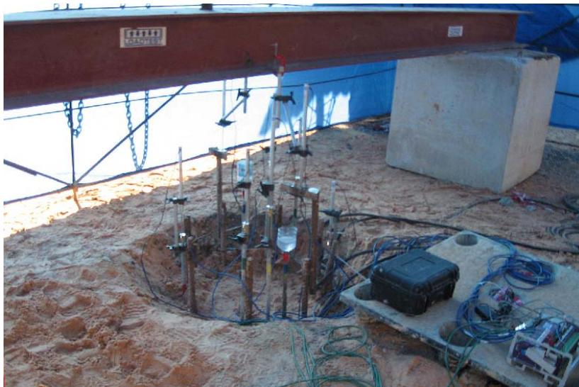
**Fig. 9 Typical pile head arrangement for a bi-directional test
