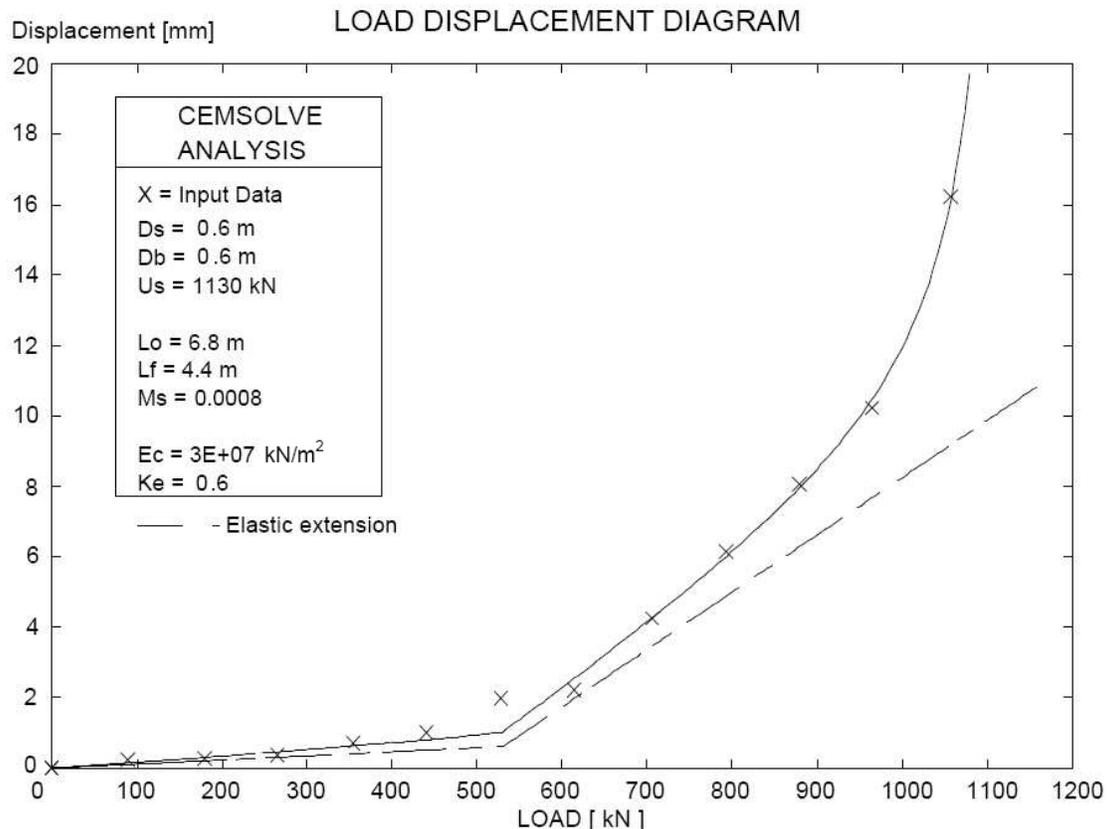
**Fig. 5 Rotary bored pile 600 mm diameter — Tension test and Cemsolve Analysis**
