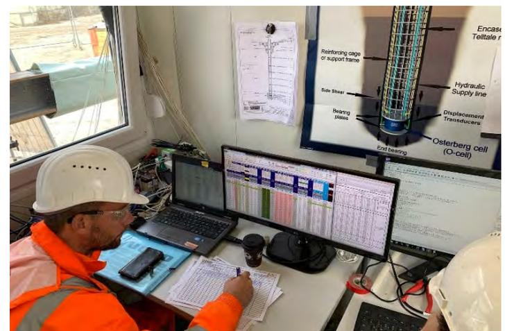
Fugro Loadtest: Static Load test in progress
