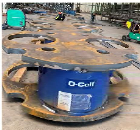
Full scale static load testing using Osterberg-cells was planned as the method is specifically appropriate for the test loads required and on piles of this size and bearing capacity. The results allow confirmation and potentially optimisation of their foundation design without the need for costly and time-consuming installation of the reaction piles used in conventional load testing.
