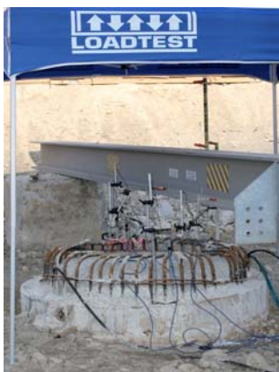
Pile head test arrangement showing reference beam during O-cell bi-directional loading in progress.
