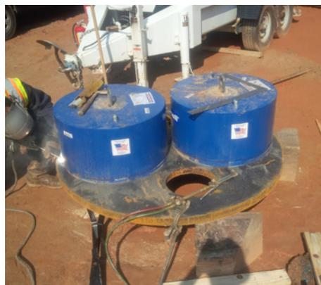
*O-Cell Load plate assembly*
