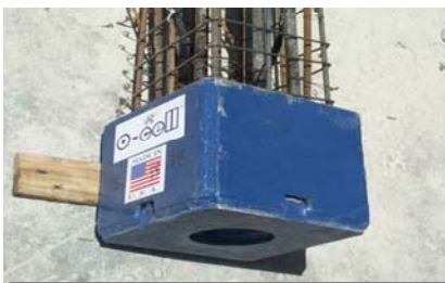
300x300mm O-cell before concreting
