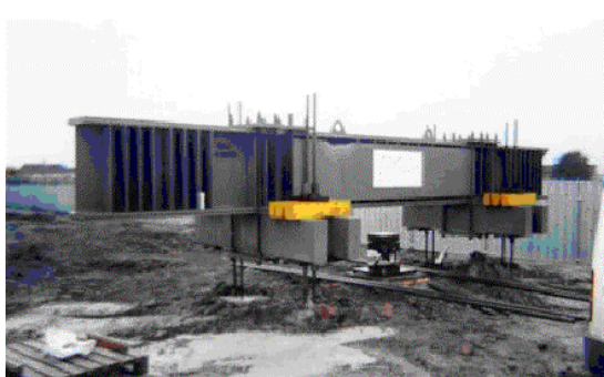
Figure 5. 5.5 MN CRAFT set up on 4 anchors with 8 Dywidag bars
