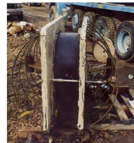
Split cylinder lateral rock modulus testing using an O-cell
