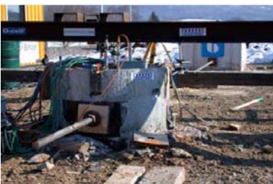
Lateral testing in progress
