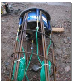
O-cell Assembly and Instrumentation
