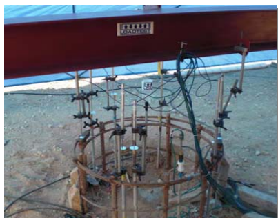
Testing in progress – pile head and reference beam
