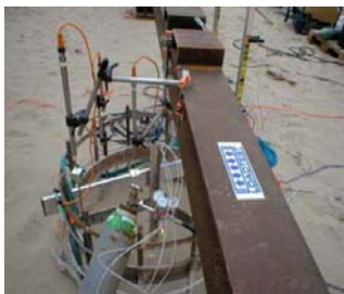
Bi-directional test in progress. Nitrogen gas is used to 'set' the A9 extensometer string
