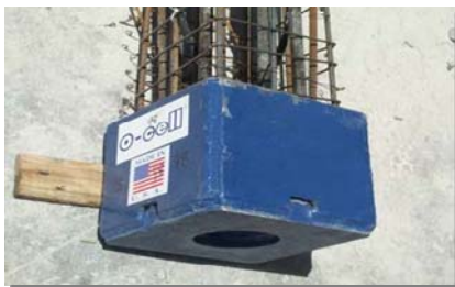
300x300mm O-cell before concreting
