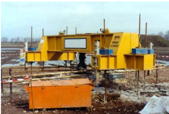
Figure 3. 2MN CRAFT set up on 6 anchors with 6 Dywidag bars
