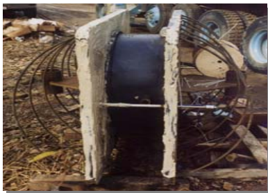
A 27MN (6000 kip) O-cell® used to test a 1500 mm (5') long by 1200 mm (4') diameter rock socket. Bearing plates are greased along the inside plane to facilitate concrete de-bonding
