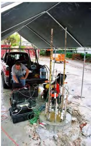
A 2,000 ton Augercast Test set up
