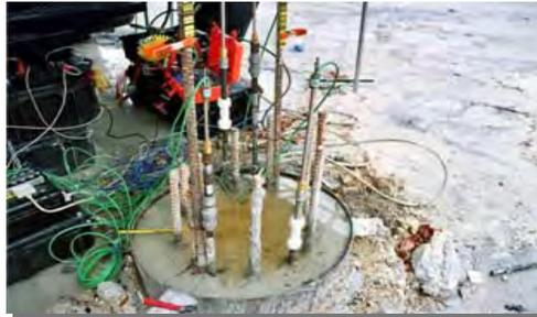
+2,000 Ton Augercast Test in progress
