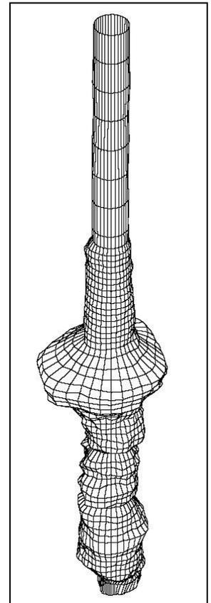
Figure 7. Rendering of Pile Shape (LOADTEST, Inc.)
