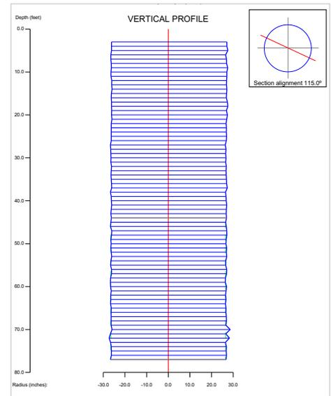
Figure 4 – SONICaliper profile – grout monitoring
