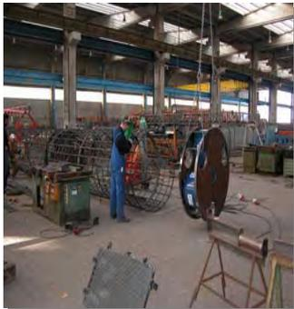
Cage and O-cell assembly fabricated off-site
