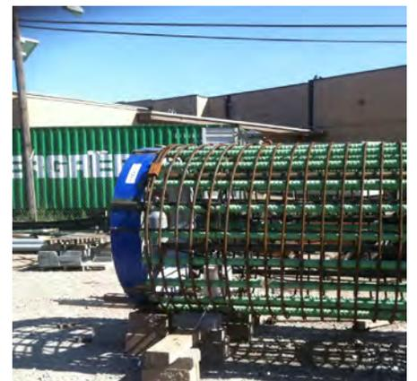
*RIM-Cell mounted on a reinforcement cage to perform a service load verification*
