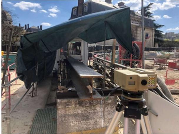
Fig. 6. Testing underway, footprint is the same as the foundation element. The beam is for datum reference only.
