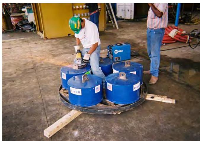
Fig 2 Assembly of multiple O-cells
