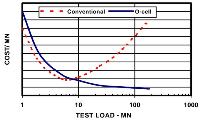
As the number of bi-directional tests increases, the costs of transportation and mobilization of personnel are appreciably reduced.
