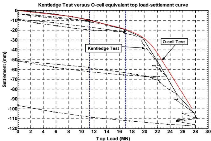
Fig 3 Comparison between top down and bi-directional
