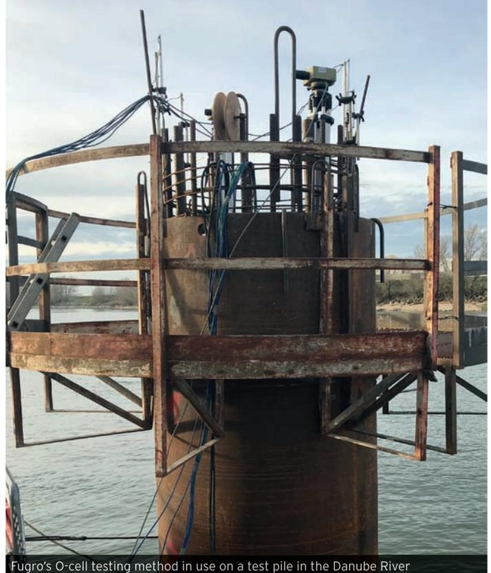
Fugro's O-cell testing method in use on a test pile in the Danube River
