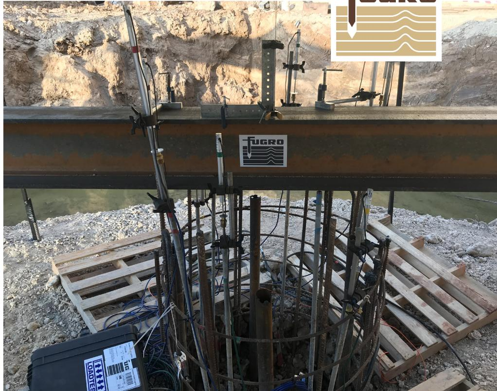
Testing under way with reference beam system to determine pile head movements.
