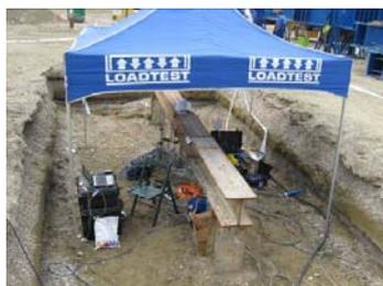
Bi-directional testing setup in Hungary
