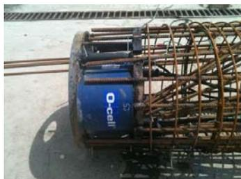
Assembly of 2x405mm O-cells placed at the bottom of a Ø1000mm pile, mobilising 24MN near Bucharest
