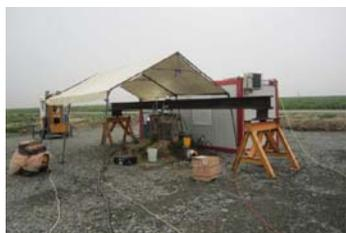
Typical bi-directional testing setup
