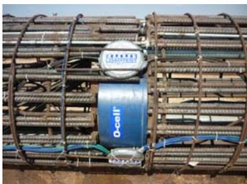
Pile reinforcing cage with O-cell instrumentation
