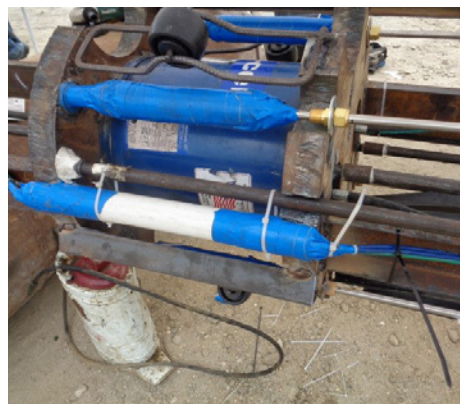
O-Cell with attached instrumentation
