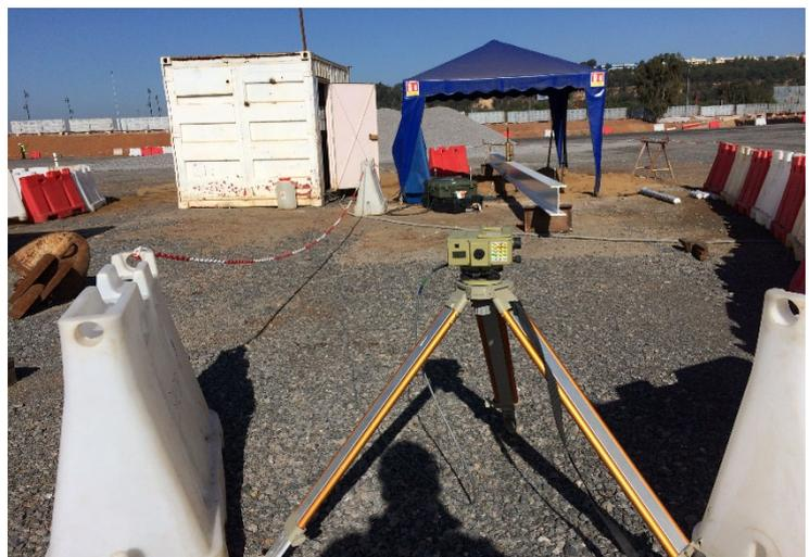
*Fugro Loadtest: Full-scale bi-directional load test in progress*
