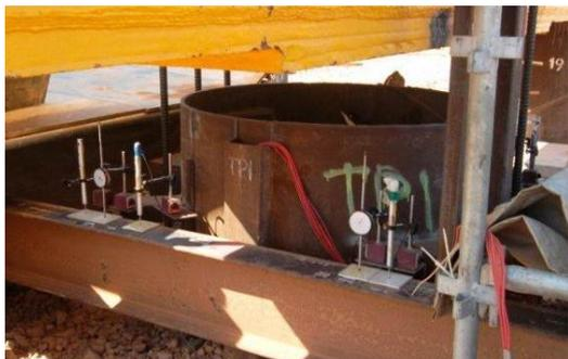
*Typical Setup of Displacement Gauges*
