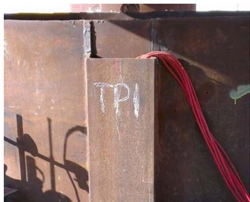
Strain Gauge Protection Channel
