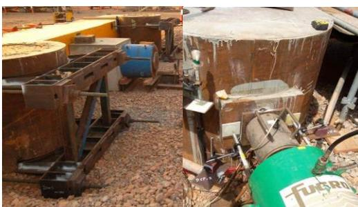
*Lateral Load Test Setup*
