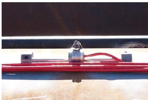
Strain Gauges Fixed To Test Piles
