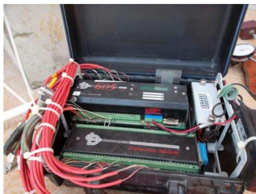
*Strain Gauge Leads Connected To Data Logger*
