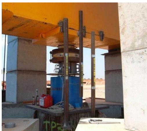
Arrangement of Jack and Load Cells
