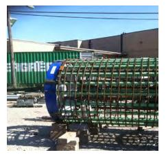
RIM-Cell mounted on a reinforcement cage to perform a service load verification
