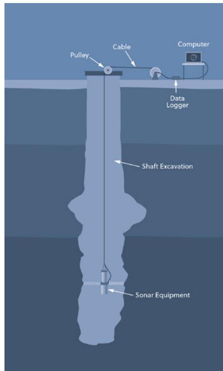
The SONICaliper determines shaft dimensions, shape, alignment and verticality.
